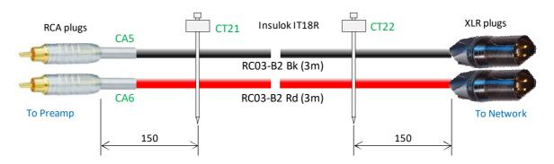
(2) Tie cable assys CA5-6 with cable tie CT23-30 at intervals of  $300\,\mathrm{mm}$ .
