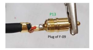
(5) Solder the white wire and shield to the cold terminal, and crimp the sheath of the cable
