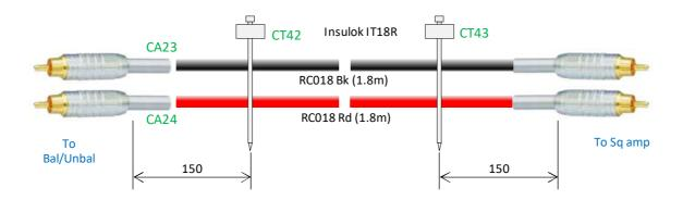
(2) Tie cable assys CA23-24 with cable tie CT44-47 (Insulok AB100-W-100) at intervals of 300mm.
