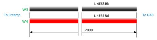
(2) Cut sleeving (FRN0.25TW) into 1.2m and slide it onto the wires (L-4E6S)
