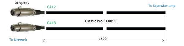
(2) Cut sleeving (FRN0.25TW) into 1.2m (SV4) and slide it onto the cabel assys CA17-18
