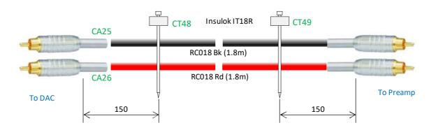
(2) Tie cable assys CA25-26 with cable tie CT50-53 (Insulok AB100-W-100) at intervals of 300mm.
