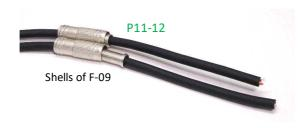
(5) Strip the insulators of the wires
