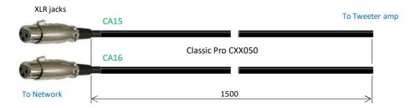
(2) Cut sleeving (FRN0.25TW) into 1.2m (SV3) and slide it onto the cabel assys CA15-16
